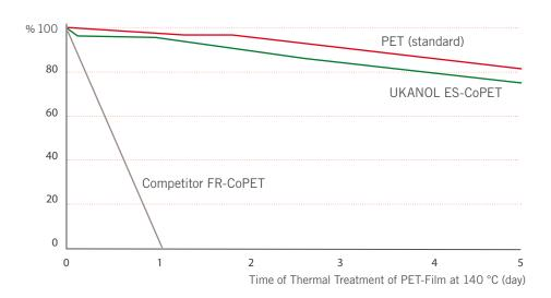
The active part of the flame retardant molecule is attached to the PET polymer chain by side chain bonding. Bond breaking by thermal rearrangement or hydrolysis in the flame retardant does not affect the integrity of the PET polymer itself. The unique characteristics of Ukanol ES-CoPET provide a fibre with hydrolysis resistance and thermal stability to match standard Polyester fibre.
