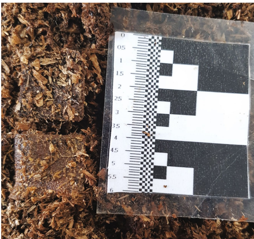
Figure 4. Photo of disintegration of triose tanned leather on day 11 of the ISO 20200 test.
